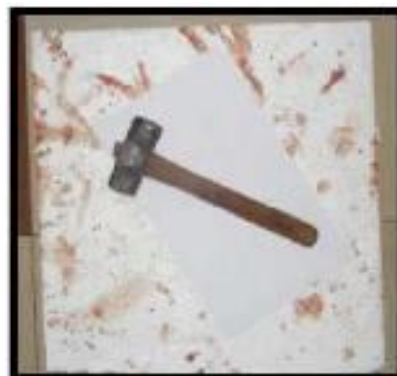
Fig. 2. Thermocol sheet placed on the floor to avoid damage of the floor tiles. Paper sheet is placed on the thermocol sheet and hammer is dropped on the paper sheet by measuring the fall height from the top of the thermocol sheet. The fall height was measured from the top of the thermocol sheet. In the next part of the experiment, each hammer was again used for 10 head hits, then dropped in a 30cc. blood pool, picked up and again made to fall from a height of 40 cms, 60 cms, and 80 cms
